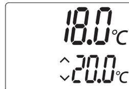
**When the wireless remote controller is installed on a bracket, room temperature might not be accurate being affected by the wall temperature. Perform a test run and place the remote controller where the room temperature can be correctly detected.**
